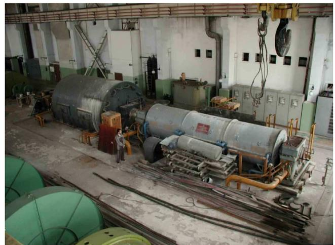
Fig. 7. FESS also known as AC Flywheel Generator used in Ukraine for operation of Stellarator power source. FESS is rated for 0.8 gigajoules of energy and maximum power delivery at 200 megawatts. For scale note the person standing near the center junction point of the flywheel and motor/generator connection [22].
